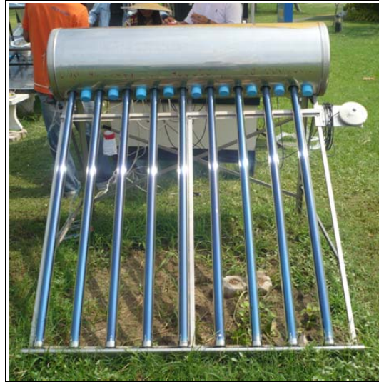
Figure 3. Evacuated tube solar hot water system without compound parabolic concentrator (Non-CPC)
