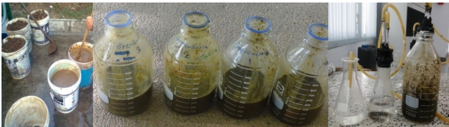
Figure2: Cow dung used as the inoculum of the digester at the started up of system
